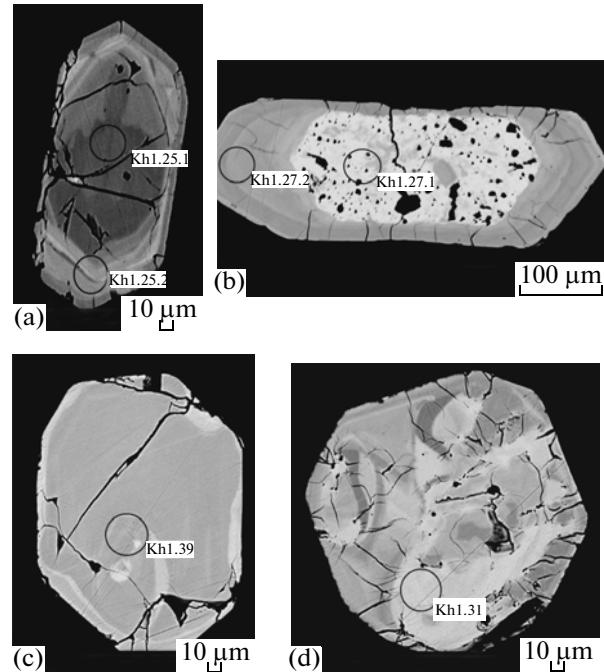
**Fig. 2.** BSE images of the analyzed: zircons of types I (a, b) and II (c, d) from sample H-1. Numbers of the analyzed points correspond to those in the table.
