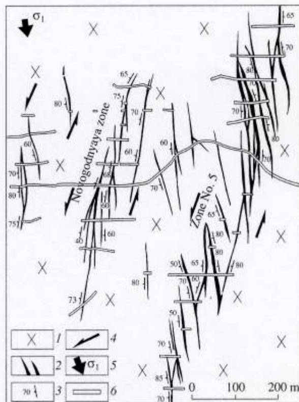
Fig. 4. Structural-dynamic formation settings of the Yagodnoe deposit. (1) Granodiorites; (2, 3) orebodies and their orientation, respectively; (4) direction of displacements with the formation of potential strike-slip faults; (5) regional compression direction; (6) exploration trenches.
