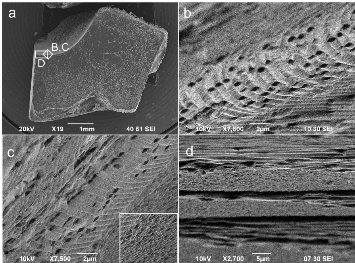
Figure 3. The EM JSM-6490LV images of hydrothermal noble opal: a – general view of the sample; b - tubules; c and d - lateral side of the layered block, the combined image of the same place made at different depth of sharpness. Top of the sample is polished, lateral sides are natural chips.
