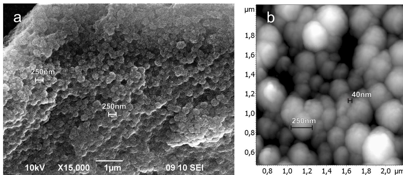
Figure 1. Supramolecular hydrothermal noble opal images: a- layers of flattened globules under EM JSM-6490LV, b- internal structure of globules under AFM Solver NT-MDT.
