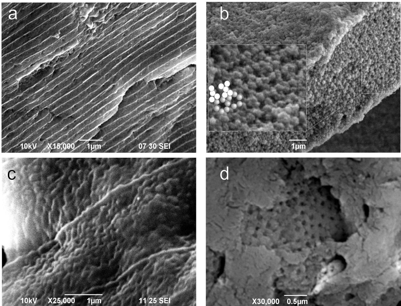
Figure 2. The EM JSM-6490LV images of layers-grids in hydrothermal noble opal: a- layered clusters, b- fragments of cubic and hexagonal pack (cutoff), c- singular layers-grids in chaotically packed opal globules, d- singular layer-grid is apparent in the "window" of randomly packed opal matrix.
