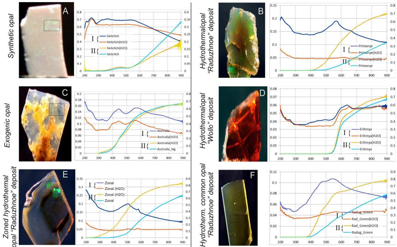
Fig. 4. Reflectance (I) and transmittance (II) spectra of the dried opals (solid line) and opals saturated with water (dashed line), Hitachi U-3010.
