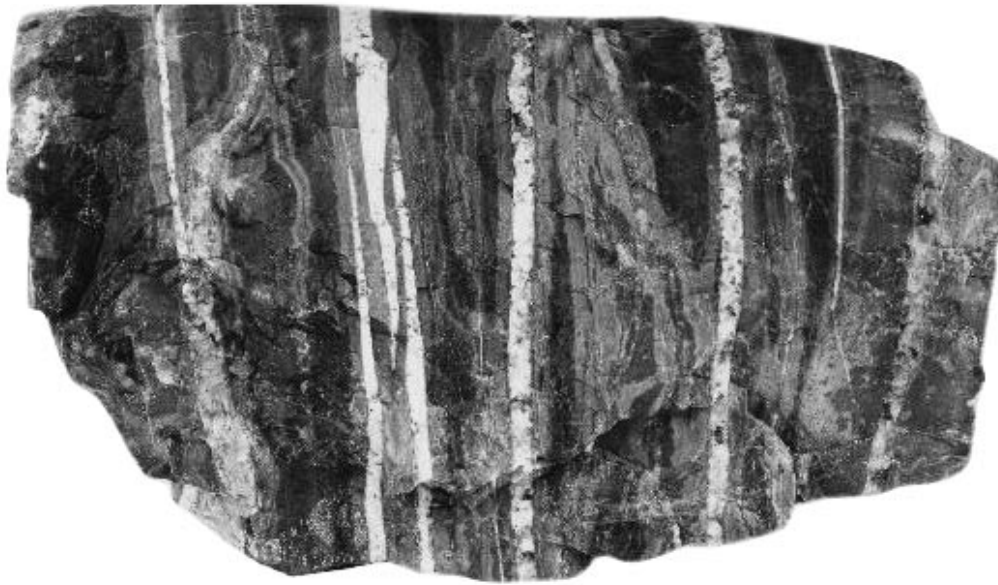
Fig. 6. Quartz–feldspar and quartz–topaz–fluorite veins and veinlets in quartz–siderophyllite hornfels are accompanied by bleaching zones. Test pit, 1/4 natural size.
